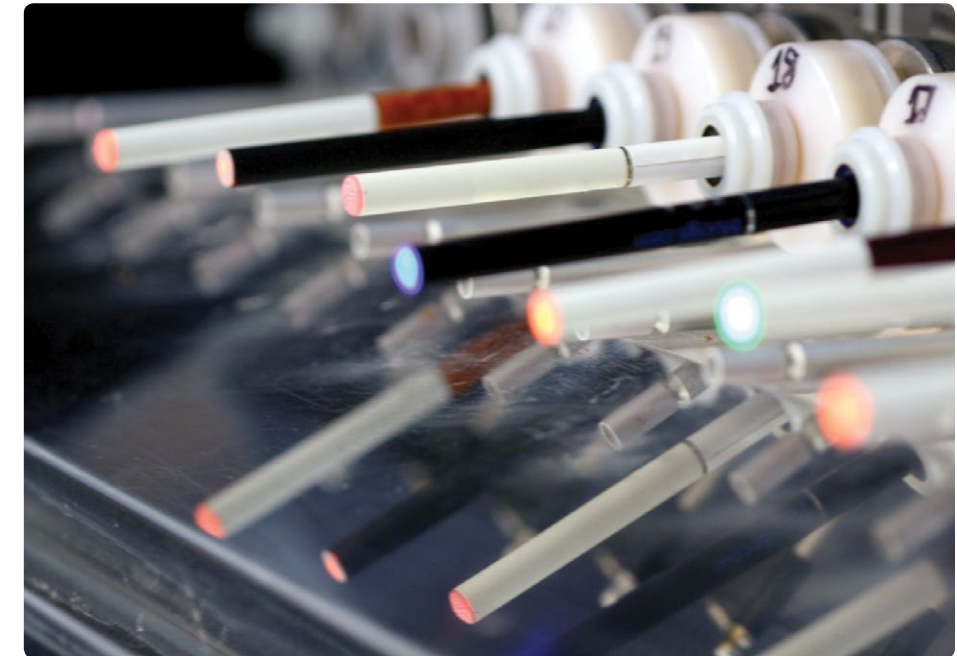
Among Enthalpy's instruments is a Linear Smoking Machine capable of simultaneously smoking twenty e-cigarettes.
